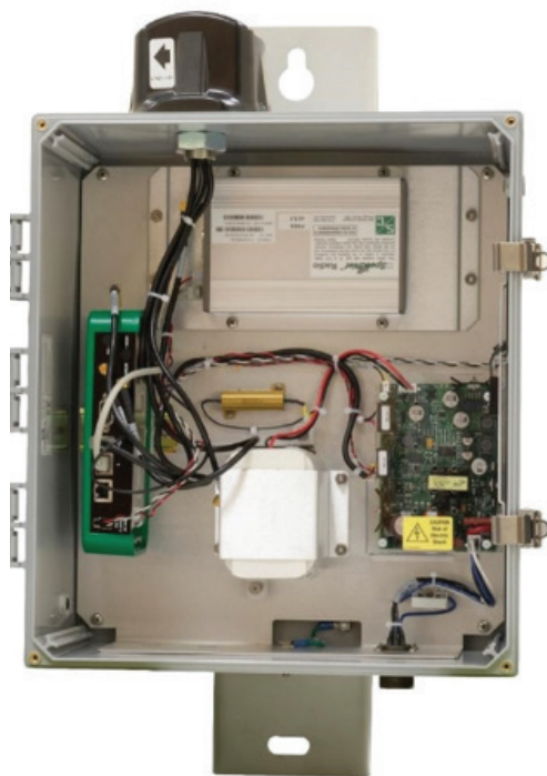
Figure 6. TripSaver II Communication Gateway
