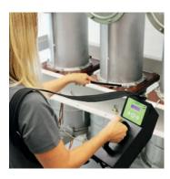
The measuring sensor extension (included in the scope of supply), which can be installed between the device and the measuring sensor, if necessary, allows measurements on measuring points difficult to access.
