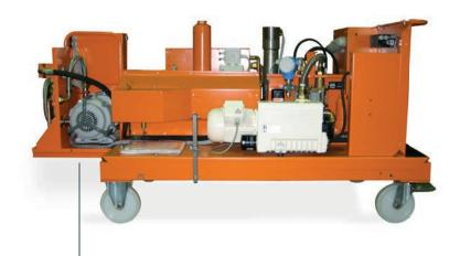
Retrofit kit for the gas recovery (suction pump) < 1 mbar
