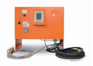
For the measurement, the gas compartment is equipped with two partially separated couplings. The gas is taken from one of the two couplings, temporarily stored in the internal gas collecting bag of the gas monitoring system and then pumped back into the gas compartment through the second coupling after the measurement has been taken. Alternatively, the gas outlet coupling of the device can also be connected to an external vessel where the gas is collected after the measurement.
