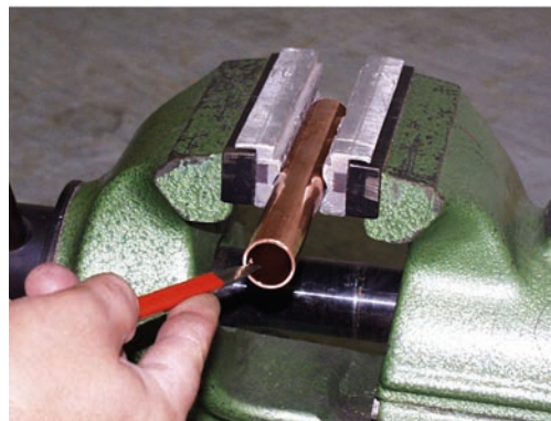
2. Deburring of the pipe extremities inside and outside
