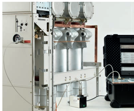
The diaphragm compressor is connected between the medium voltage breaker and the measuring device by means of the corresponding connecting hose.
