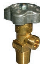
Valve for new SF 6 * as well as used SF 6 with a SO 2 content of < 250 ppm v in accordance with DIN 477 no. 6 W21.8 x 1/14" Brass
