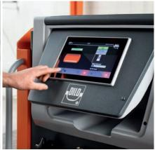
Operation, indication of the important process parameters and illustration of the selected gas flow on the touch panel. Indication units (e.g. bar/mbar/kg) can be selected directly on the panel.
