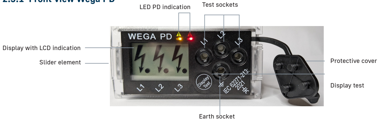
Fig. 2.2: Front view Wega PD with indications and controls
