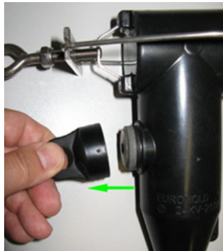
Fig. 4.1: Removing the cover cap, screw and washer
