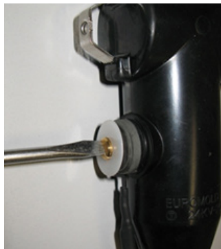
Fig. 4.2: Connecting the coaxial cable
